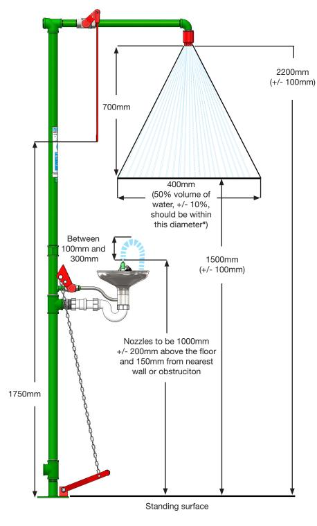
\*The area reached by a minimum of 95% of the water should not exceed 800mm in diameter.
